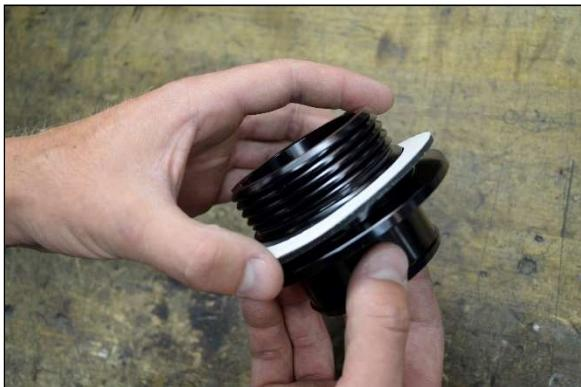
Step 16: Peel off backing on other side of rubber seal & install exhaust outlet from inside of hull. Install lock nut removed on step 13 onto billet exhaust outlet.
