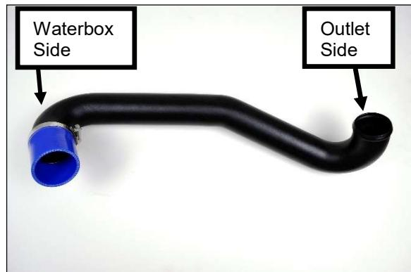
Step 19: Loosely place supplied hose clamp over reduction coupler at exhaust outlet. Loosely place other supplied hose clamp over waterbox outlet. Place free flow tube in position, connecting waterbox to exhaust outlet. Secure free flow tube by tightening hose clamps. **Do not overtighten clamp.** (See illustration below.)
