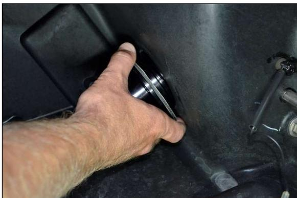
Step 17: Install supplied 2.25" x 2.5" reduction coupler on billet exhaust outlet. Apply glass cleaner to the inside of the coupler to ease installation. Use supplied hose clamp to secure. **Do not overtighten clamp.**
