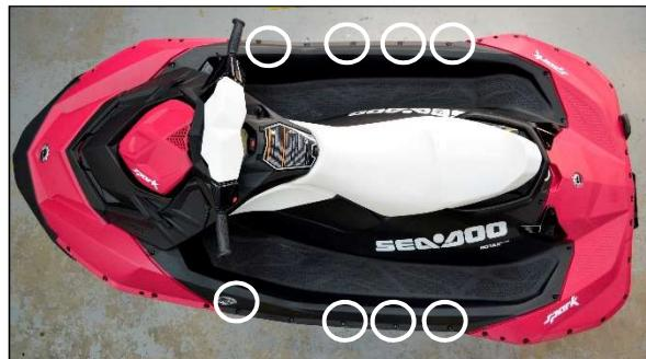
Step 24: Reinstall rear trim pieces (refer to step 8) & reinstall self-tapping screws at front & back of hull. (Circled in illustration below.) Torque to 5.5 Nm / 49 inch lbs.
